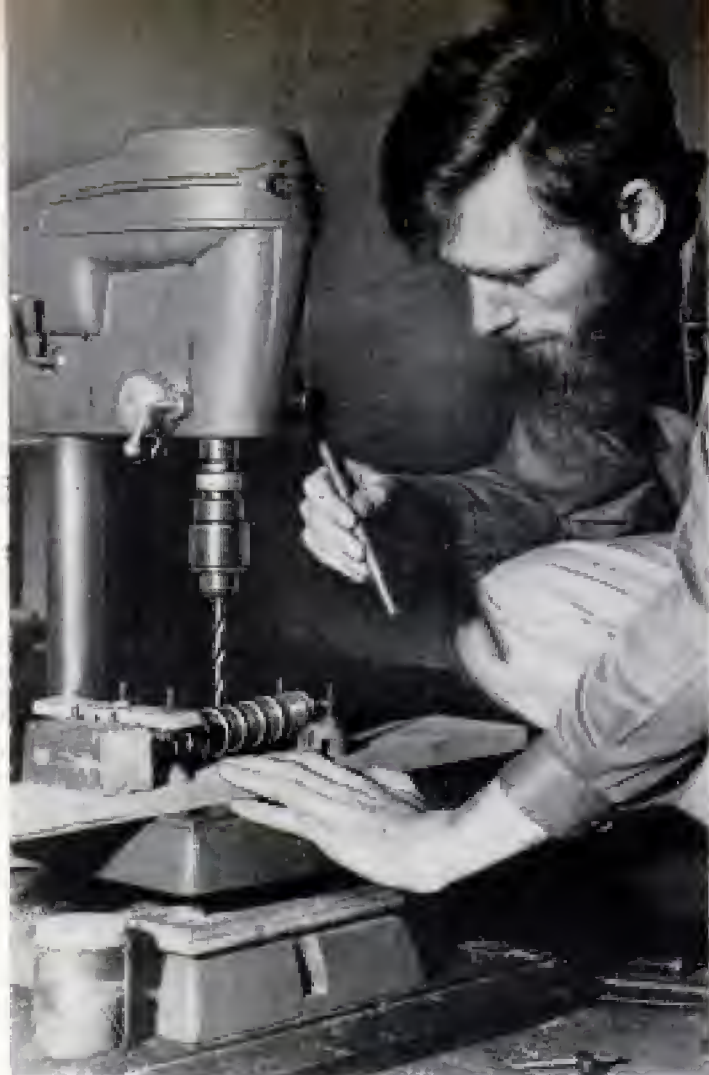
Next, Herd drills holes in the barrel for inserting the trunnions, the pins on which the barrel pivots
